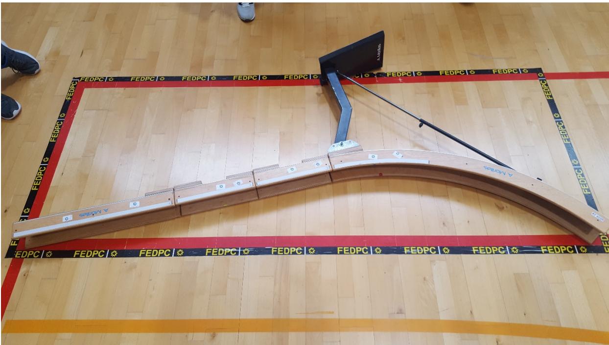
Photo #2 Assistive Devices Test: However, when the support bar is completely extended as stated in Rule 5.1, the ramp is not legal. The support bar must be cut so the ramp may not fully extend which would make this ramp illegal.
