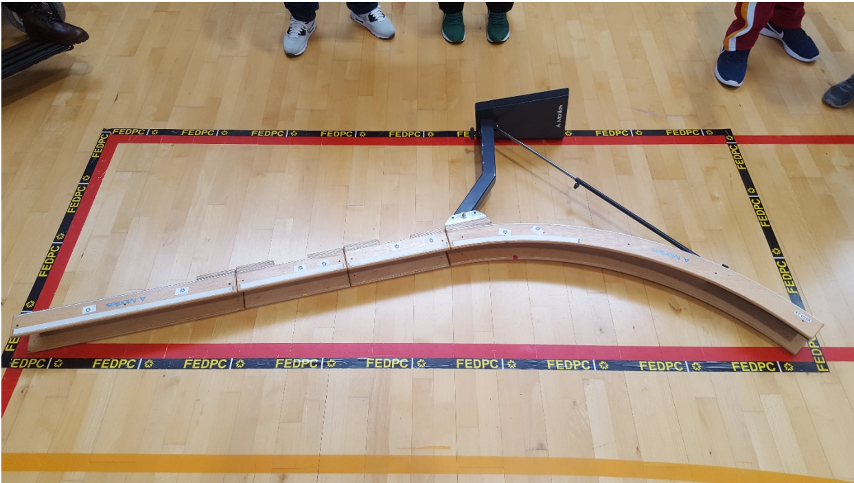
Photo #2 Assistive Devices Test: However, when the support bar is completely extended as stated in Rule 5.1, the ramp is not legal. The support bar must be cut so the ramp may not fully extend which would make this ramp illegal.
